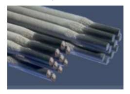
**Description:** A rutile coated electrode-depositing air hardening type weld metal of appox. 250 VPN hardness. The electrode is having excellent operating characteristics like smooth and steady arc, easy striking and restriking, superior bead finish and easy slag detachability. The electrode can also be used easily in positions. The weld deposit is machinable with normal tools. Weld metal has good abrasion and impact resistance.
