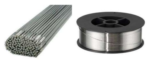
Three common forms of filler wires are metal-cored, flux-cored, and solid wires. Copper coating is commonly used on solid wires to prevent oxidation, improve electrical conductivity, and extend the lifespan of welding contact tips. Flux-cored wires employ an electric arc fuse to link two pieces of metal. These wires shield the welds from contaminants and oxidation. Metal-cored wires are tubular
