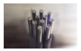
**Description**: A rutile coated electrode for welding of general structures under static loading to moderate dynamic loading conditions. The electrode is having a balanced arc, which ensures good penetration under any condition. The slag is quick freezing and easy to control. The electrode is highly tolerant to rusty plates and poor fit -ups.
