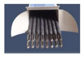
**Description:** A specially formulated electrode with phosper bronze core wire for welding of copper and copper alloys like brasses and bronzes. The electrode is having good operating characteristics and is capable of welding in positions. The weld deposit is machinable.
