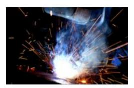
**Description:** A medium coated specially formulated low heat input electrode for welding of mild and medium tensile steels. The electrode operates with a smooth arc, minimum spatter and reduced current. The electrode works with ease in all positions. The slag is easily detachable and the deposit is of radiographic quality.
