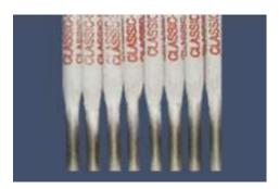
**Description**: A heavy coated basic iron powder type low hydrogen electrode for welding of weathering steels, medium and high tensile steels and joining them to mild and other structural steels. The electrode is having very good operating characteristics like smooth and steady arc, slag detachability. The electrode can be used easily in positions. Weld deposit is of high radiographic soundness.
